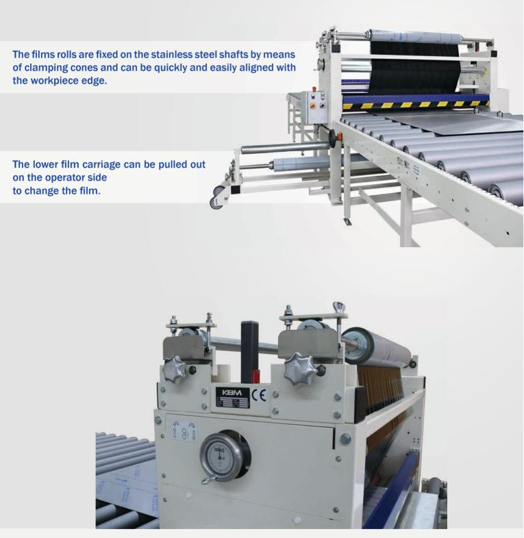
The film is pulled from the roll via a deflection roller and the film tension can be adjusted by means of a finely adjustable brake. The workpiece thickness is set via the handwheel with passage height indicator.
